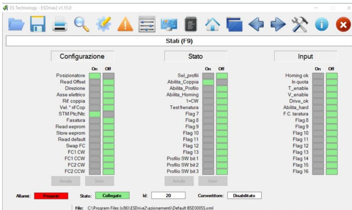
When the "**Positioner**" mode is selected, when the converter is switched on, the auxiliary digital input 2 is used as an end of stroke to search for the position of zero. The limit limit is considered reached when there are 0V for at least 100ms on the corresponding clamp.
