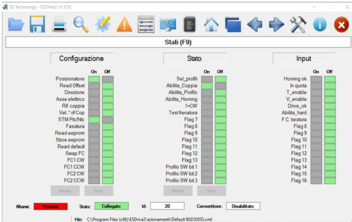
Once you have selected the desired bit configuration, you must send it to the converter using the **Out** button. The **In** key is used to read the configuration of the drive in case the automatic reading is disabled.
