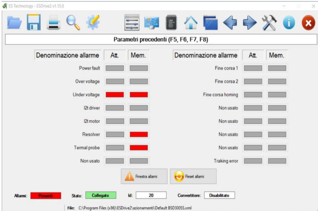
All alarms except the Power fault reset automatically. The Power fault needs to turn off the converter to be reset.
