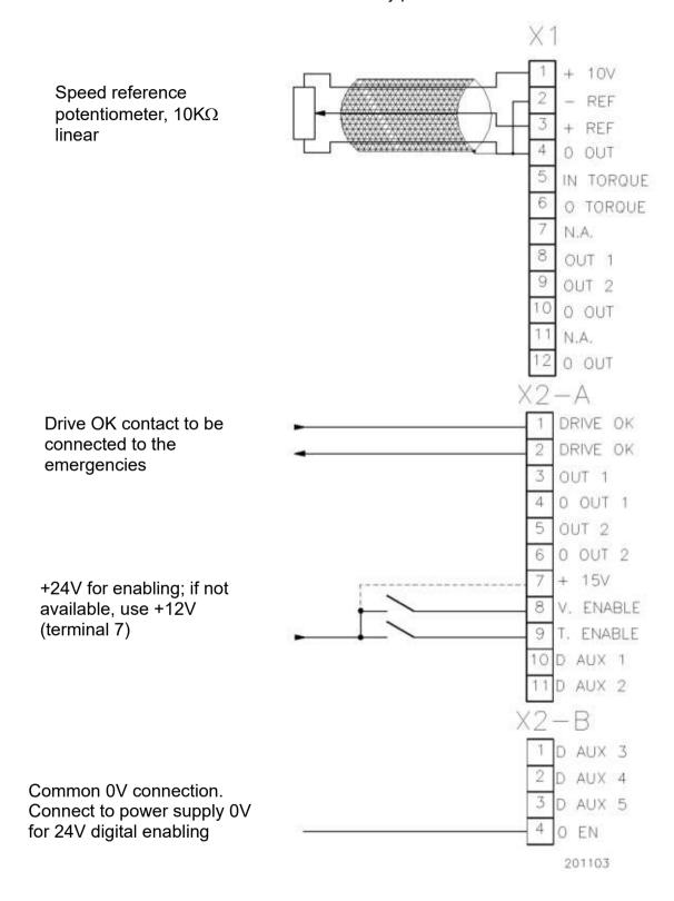
**4.2 Connectors X1 e X2:** Connection with reference by numerical control and reading by encoder simulator
