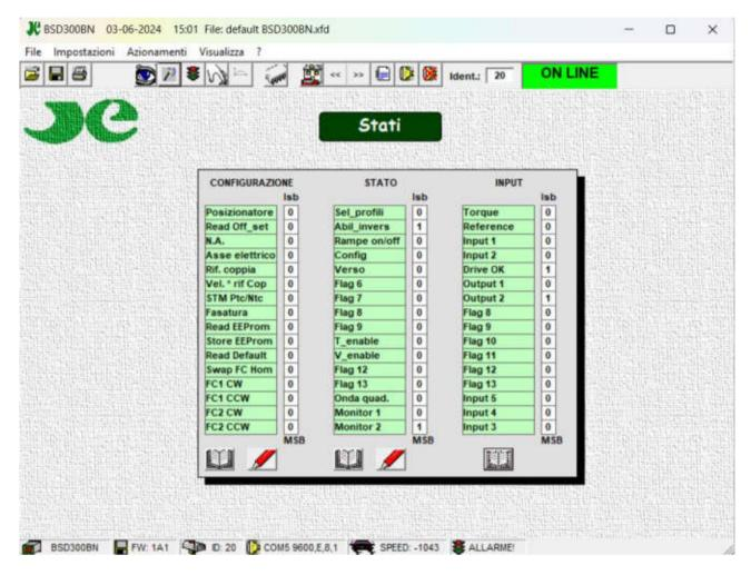
Once the desired bit configuration has been selected, it must be sent to the drive using the **ENTER** key.
